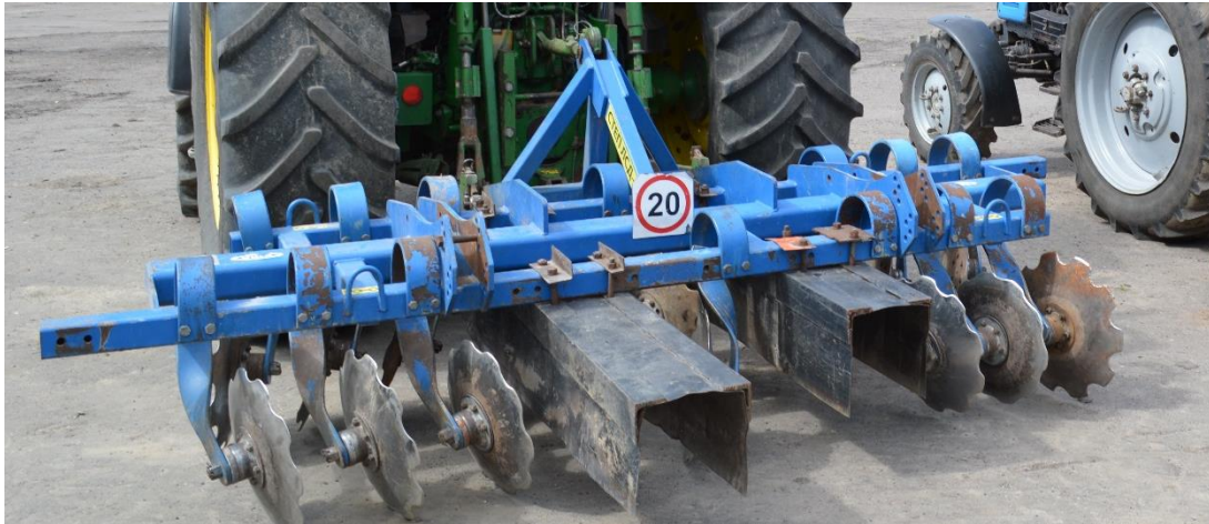
FIGURE 28. DISC PLOUGH-HARROW LSD FOR WILLOW PLANTATIONS
