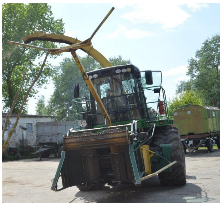
FIGURE 30. SELF-PROPELLED FORAGE HAVESTER JOHN DEERE 7300 WITH SPECIAL WODDY CUTTING HEAD HSAB'S SRC
